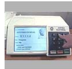
Used in Brazil for recording votes, the electronic ballot box is a small, self-contained computer and printer that stores voting data. It includes battery backup, so that votes can't be lost because of power failure.
